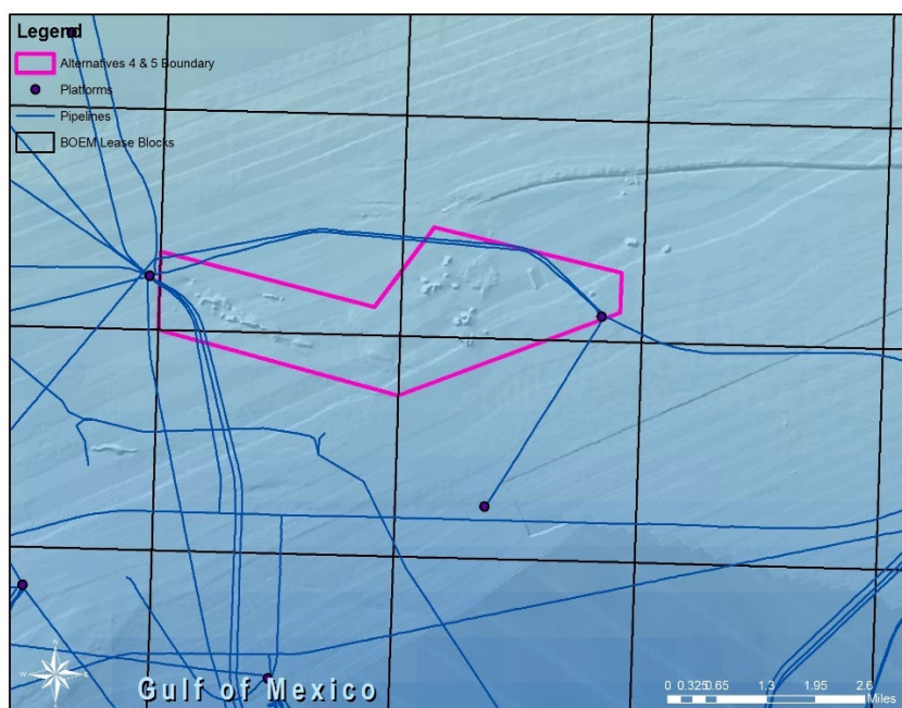
Figure D.78. Double Top boundary alternatives 4 & 5, existing regulatory zones, and infrastructure. Image: NOAA
